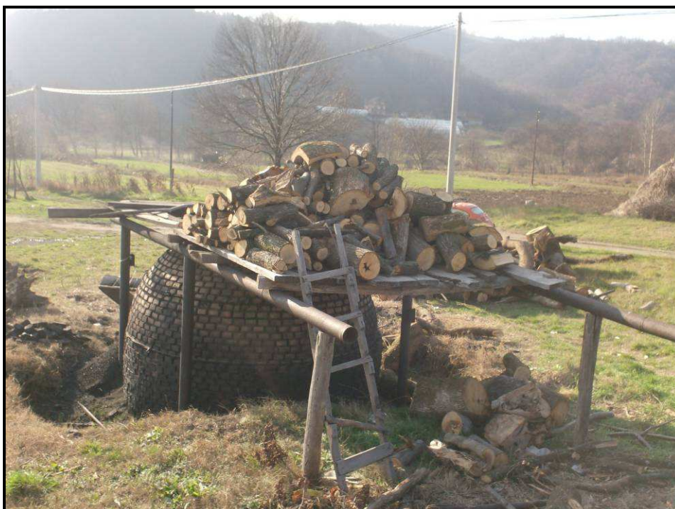
COAL PIT BUILT ON THE MAJDANPEK – BOR ROAD: PREPARED BEECH CHARCOAL TREE
